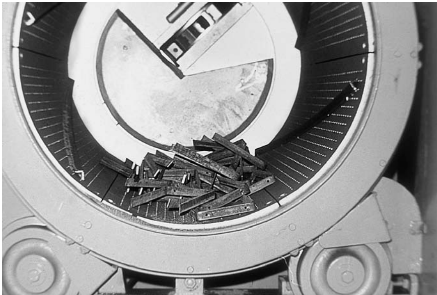
Figure 7.3 Rotating drum for diffusion process.
