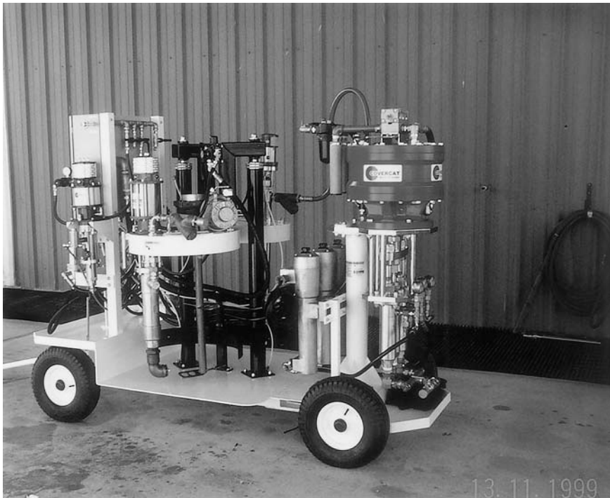
Figure 5.3 Plural system equipment for application of heated two-component coatings. Source: Covercat Spray Systems Ltd.
