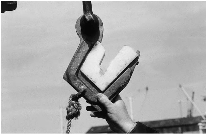
Figure 8.1 Crane hook with soft renewable contact surface to minimise coating damage.
