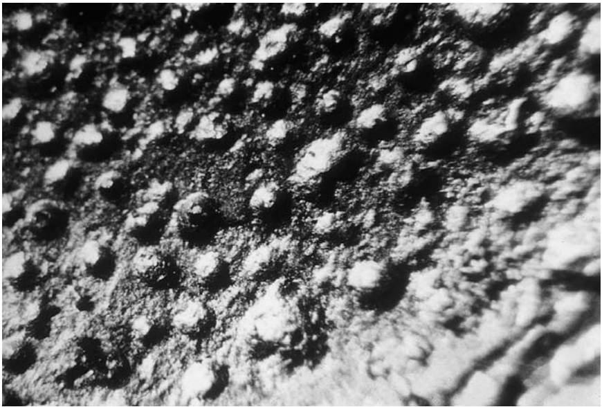
Figure 13.7 Blister from within the coating film.
